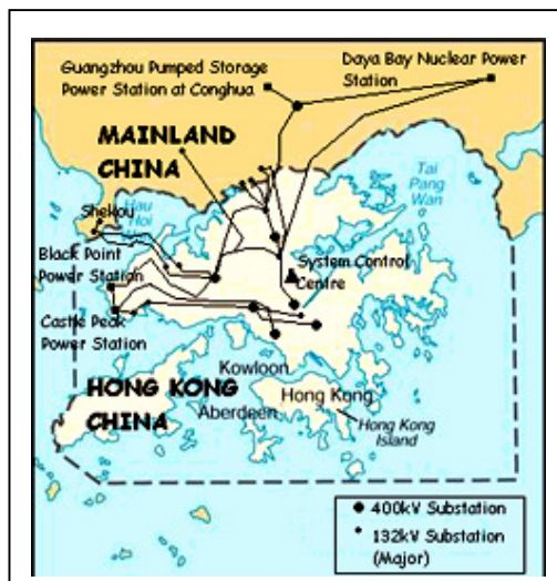
Figure 2: Existing CLP's power grid extending from the New Territories, Hong Kong, into Guangdong
