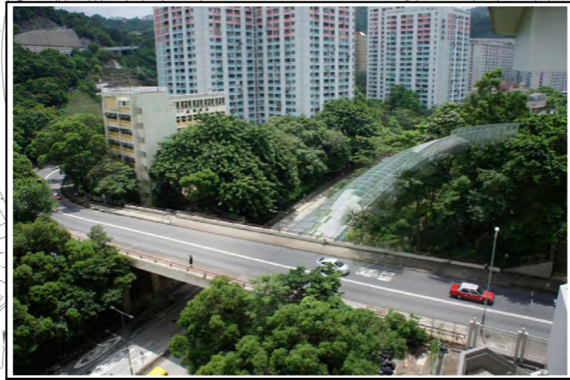
密封式隔音罩及隔音屏障模擬照片 NOISE FULL ENCLOSURE AND NOISE BARRIER PHOTOMONTAGE
