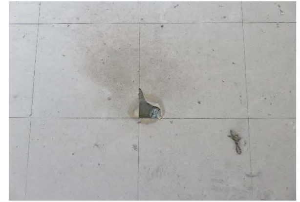
Photo 2432: S33, vinyl floor tile with mastic in bedroom of Room 9, 4/F, Quarter Block. No ACM was identified. (Lab ID: B/103/16/33)
