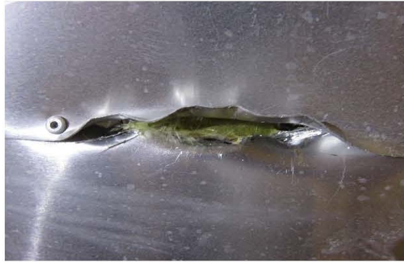
Photo 2057: Glasswool insulation of the heater under the metal casting in E&M Workshop
