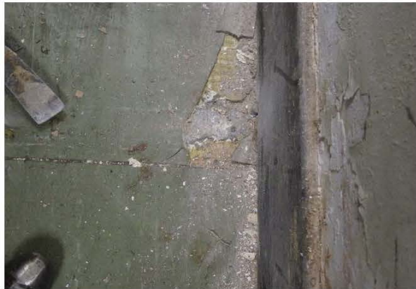
Photo 2221: S22, vinyl floor tile with mastic in Store Room, G/F, EMSD Headquarters. No ACM was identified. (Lab ID: B/103/16/22)
