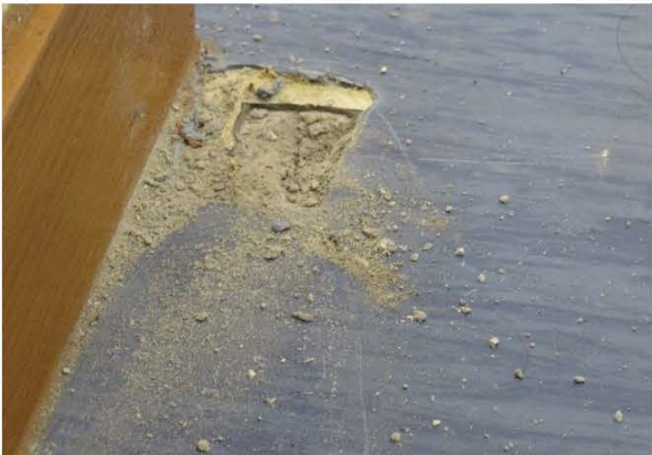
Photo 2206: S16, vinyl floor sheet with mastic on 2/F, EMSD Headquarters. No ACM was identified. (Lab ID: B/103/16/16)
