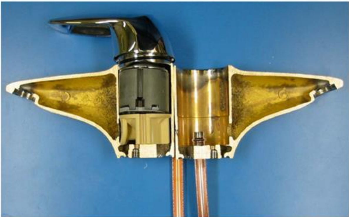
Figure 1: Example of nickel-chromium plated mixer tap. Nickel is observed at the inside of apertures.
