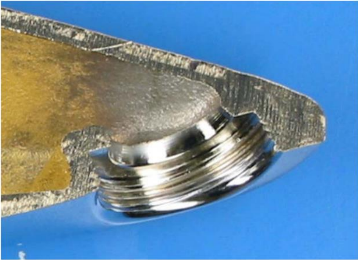
Figure 2: Close-up of aperture on mixer tap spout showing nickel at the inside.
