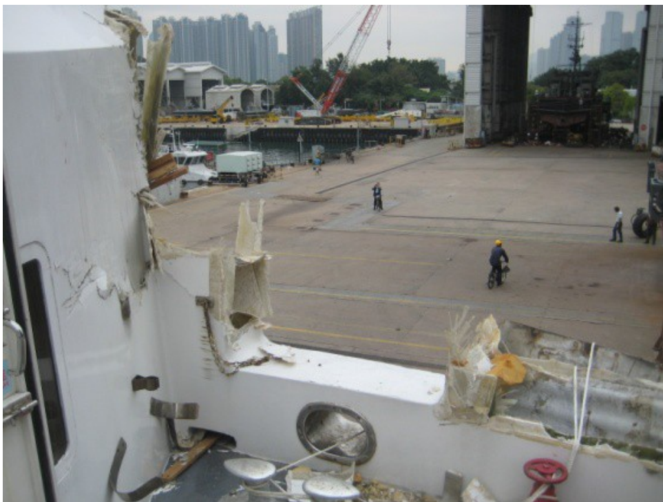
Figure 3: Photo showing the extent of damage to the part of Sea Smooth involved in the collision
