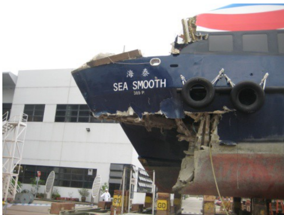
Figure 1: Photo showing the extent of damage to the part of Sea Smooth involved in the collision
