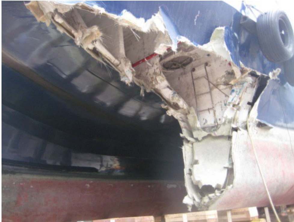
Figure 2: Photo showing the extent of damage to the part of Sea Smooth involved in the collision
