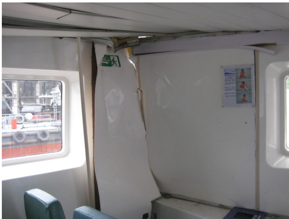
Figure 5: Photo showing the extent of damage to the part of Sea Smooth involved in the collision
